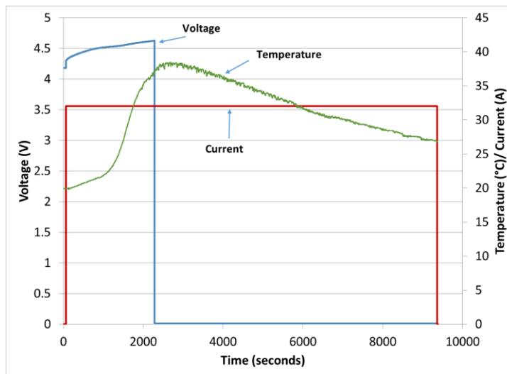
Figure 5: Results for overcharging – PDD activation test
