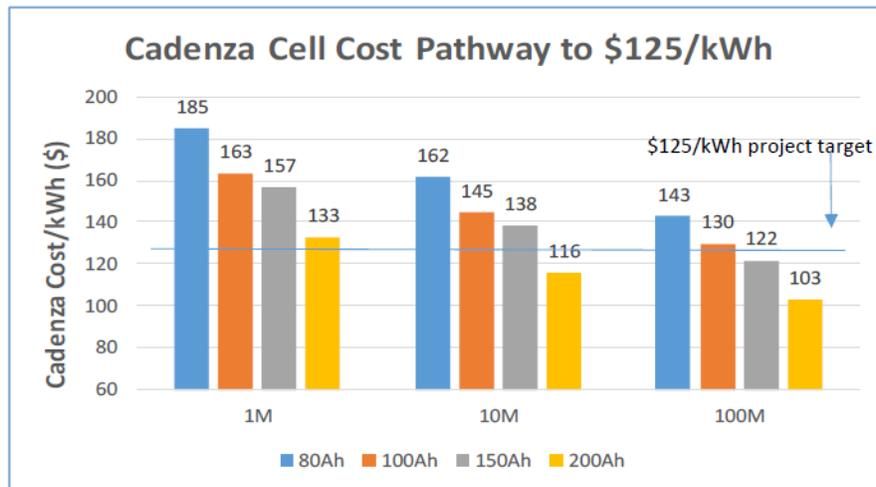
Figure 16: Manufacturing costing estimates for the Cadenza cell/platform
